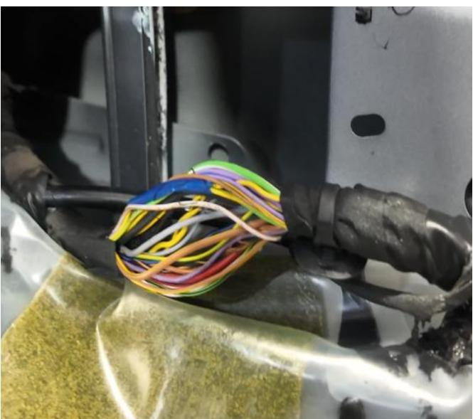
Alternatively, the connections can be made to the plugs itself which may be easier to identify. However, this will mean that some wiring will need to be extended. If you have a multimeter, verify that you are connecting to the correct wires before making connections.
